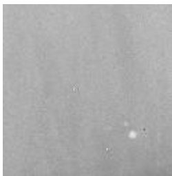
Figure 27. A radiograph of the Titan-64 wire DED-L sample, approximately 5 \times 5 \text{ mm}^2 is covered in the radiograph with an effective pixel size around 0.05 mm
