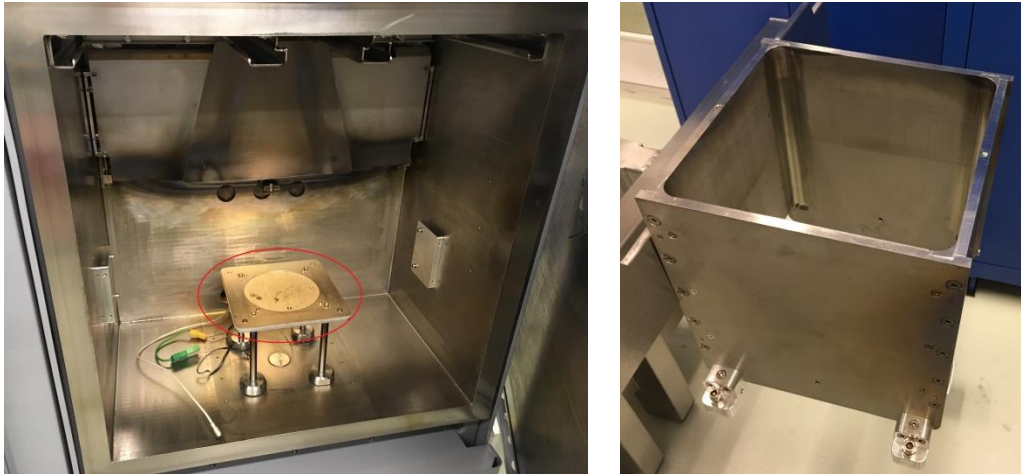
Figure 1. Photograph of the interior of a PBF-E machine from Arcam. Left) build process chamber with the build platform encircled in red, right) the build tank which is positioned over the build platform, wall thickness around 10 mm, in order to keep the powder in position.
