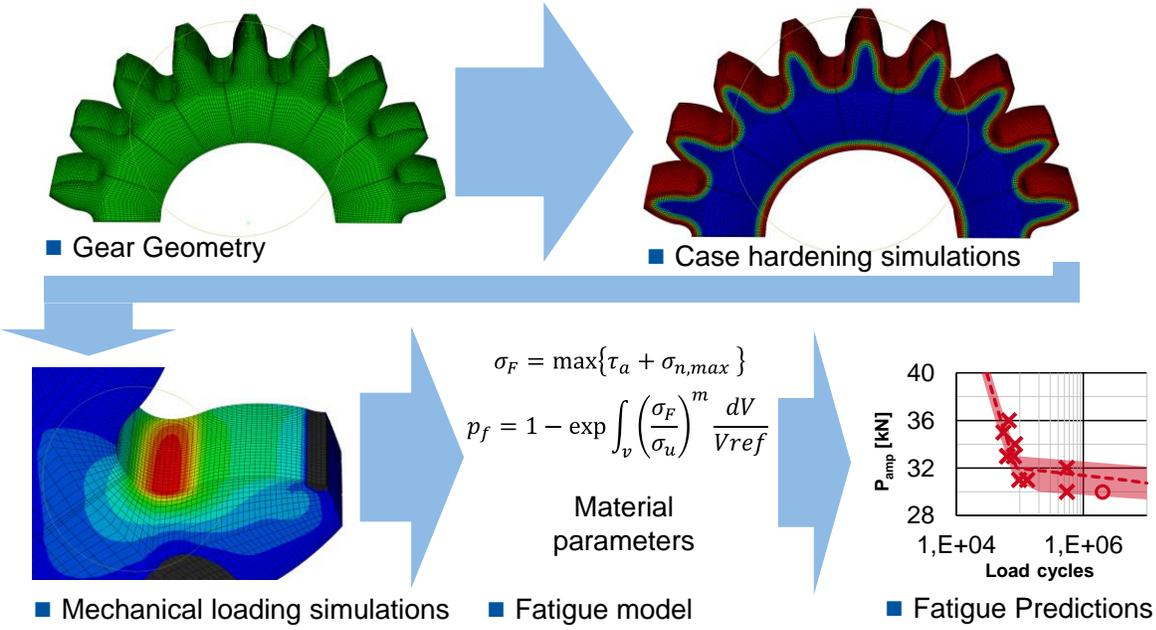
**Figure 1.** Visualization of the virtual dimensioning approach developed and used in the project.
