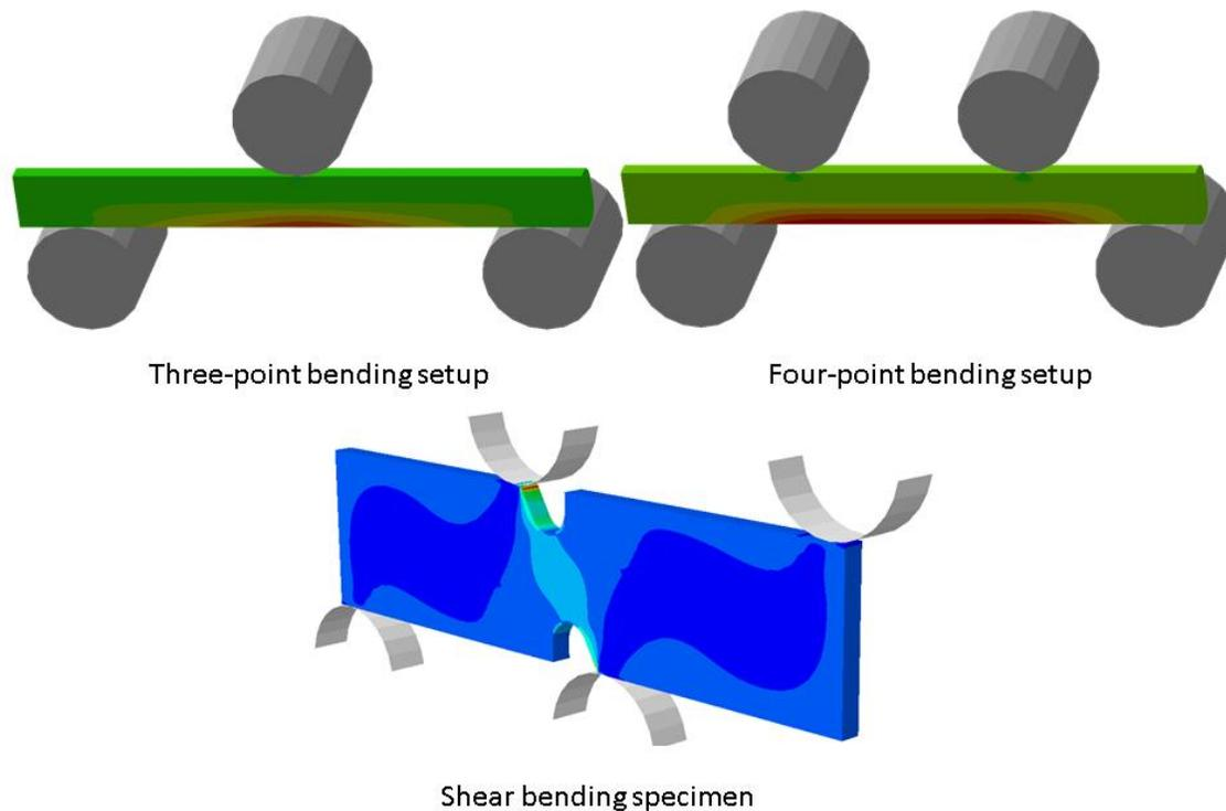
**Figure 4:** The two different fatigue specimen designs and the way they are tested.
