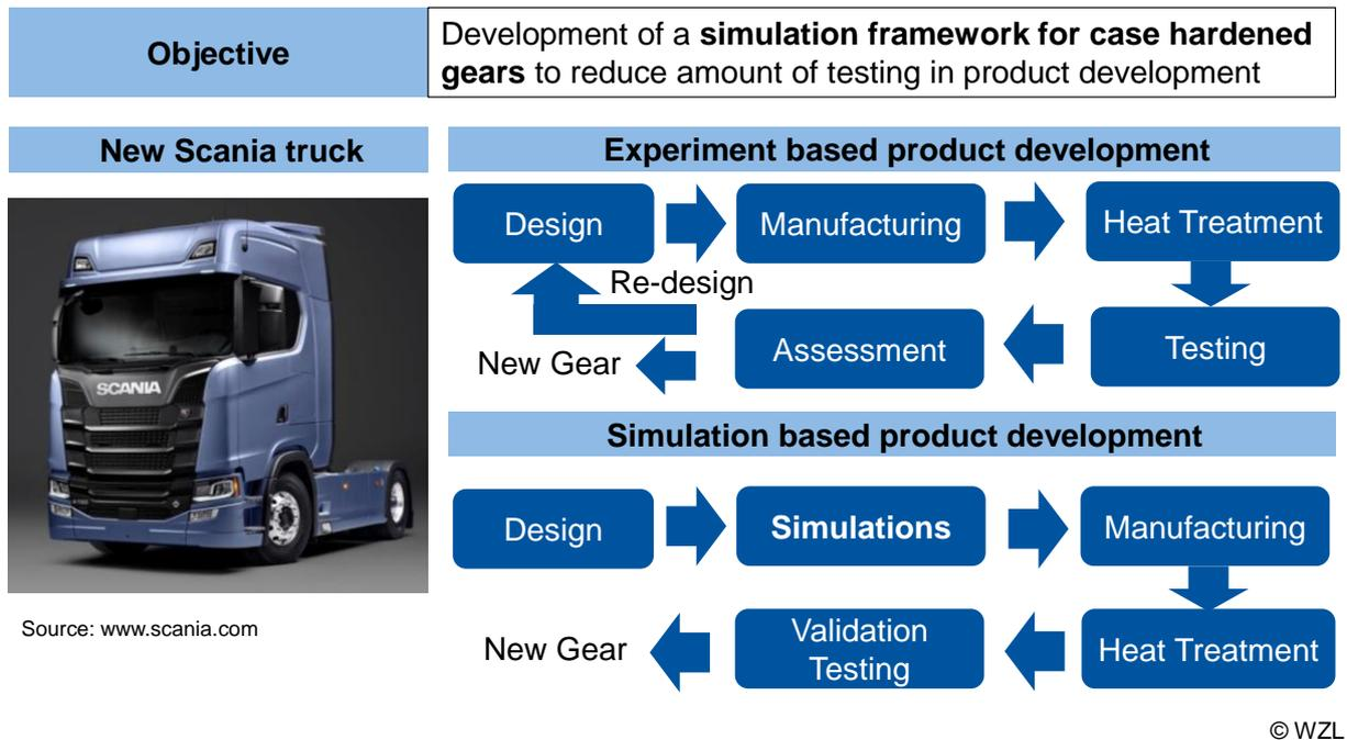
**Figure 1:** Motivation of the Work by Enabling a Simulation based Product Development of Case Hardened Gears.
