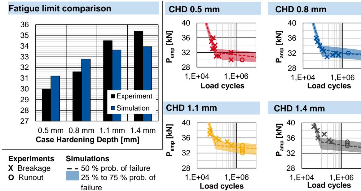
**Figure 3:** Fatigue limit and life predictions compared with experimental results.
