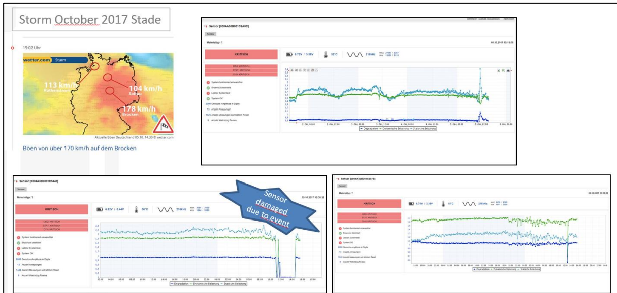
Figure L5. During a storm a tree fell on a pipe which was detected by the lamb wave sensor technology.
