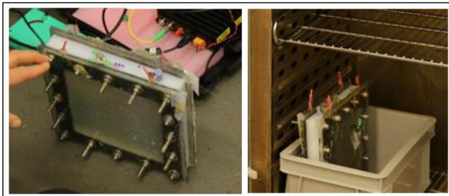
Figure 12. The experiment setup for the single sided exposure to water at 70 °C.
