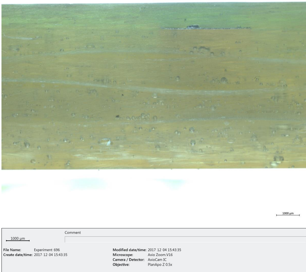
Figure 17. Microscopic picture over the cross section of the laminate with incorporated thin metal films after 90 days exposure in HCl.
