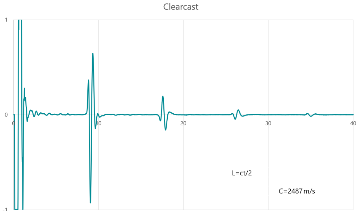
Figure 34. The echo recorded from a sample made of clear cast with no glass fibres.
