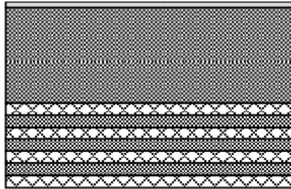
Figure 3. Schematic picture of an FRP laminate, at the top the corrosion barrier (red arrow) and at the bottom the structural bearing layer. [1]
