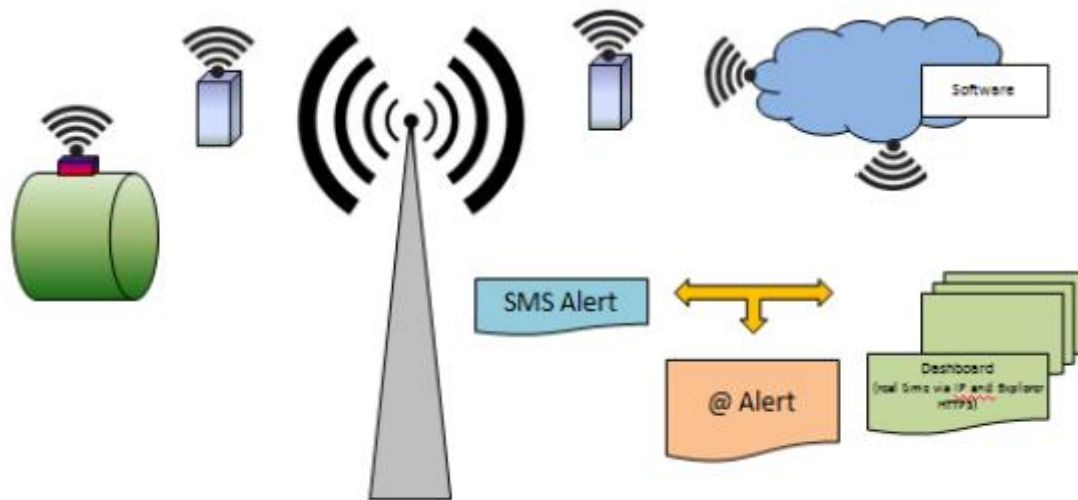
Figure L4: Smart network that enables online monitoring with a large number of installed sensors.
