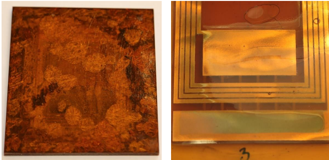
Figure Invi-7a. Sample 5 after exposure in the flue gas stack and (b) the backside of sample 3 after exposure, where it can be that the copper has turned green due to corrosion.
