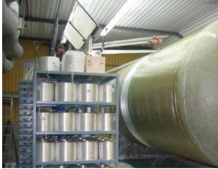
Figure 2. Manufacturing of tank in FRP made by a machine. [1]
