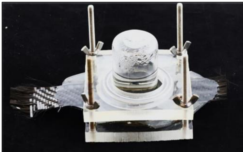
Figure 23. Single sided exposure of sample 4.
