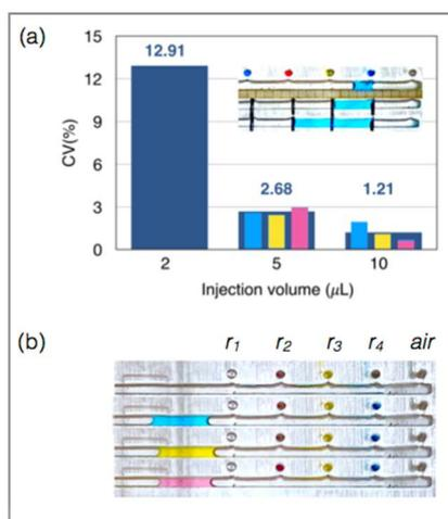
Fig. 2a) Reliability of injectors expressed as coefficient of variation for injection volumes between 2 and 10μL. b) Zoomed area on null dead volume check valves showing absence of contamination between injectors and manifold when 5μL volumes flow in the manifold.
