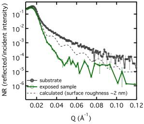
**Figure 1.** NR curves as measured on the substrate (black) and an exposed sample (green). A calculated curve for the case of a sample with low roughness (gray, dashed) is also shown
