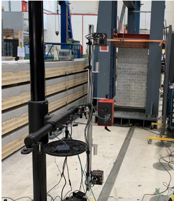
Figure 8 3D high-speed DIC measurements: View of the set-up.
