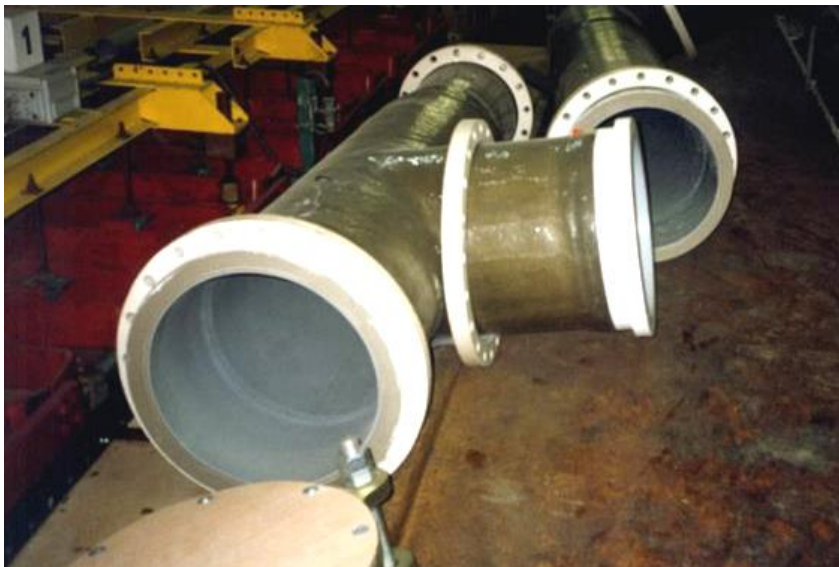
Figure 31. A CPVC/FRP pipe section for a chlorine header.
