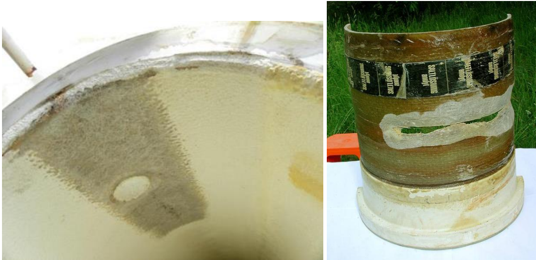
Figure 34, Two different CPVC/FRP pipes for analyte (brine with dissolved Cl_2 ) i.e. in the low pH range of the hypochlorite balance. Both pipes have regions where the flow was stagnant, and the pH increased so that HClO was formed. This resulted in rapid degradation of the material. The rest of the CPVC has been attacked but by Cl_2 but this is much less harmful to CPVC than the HClO .
