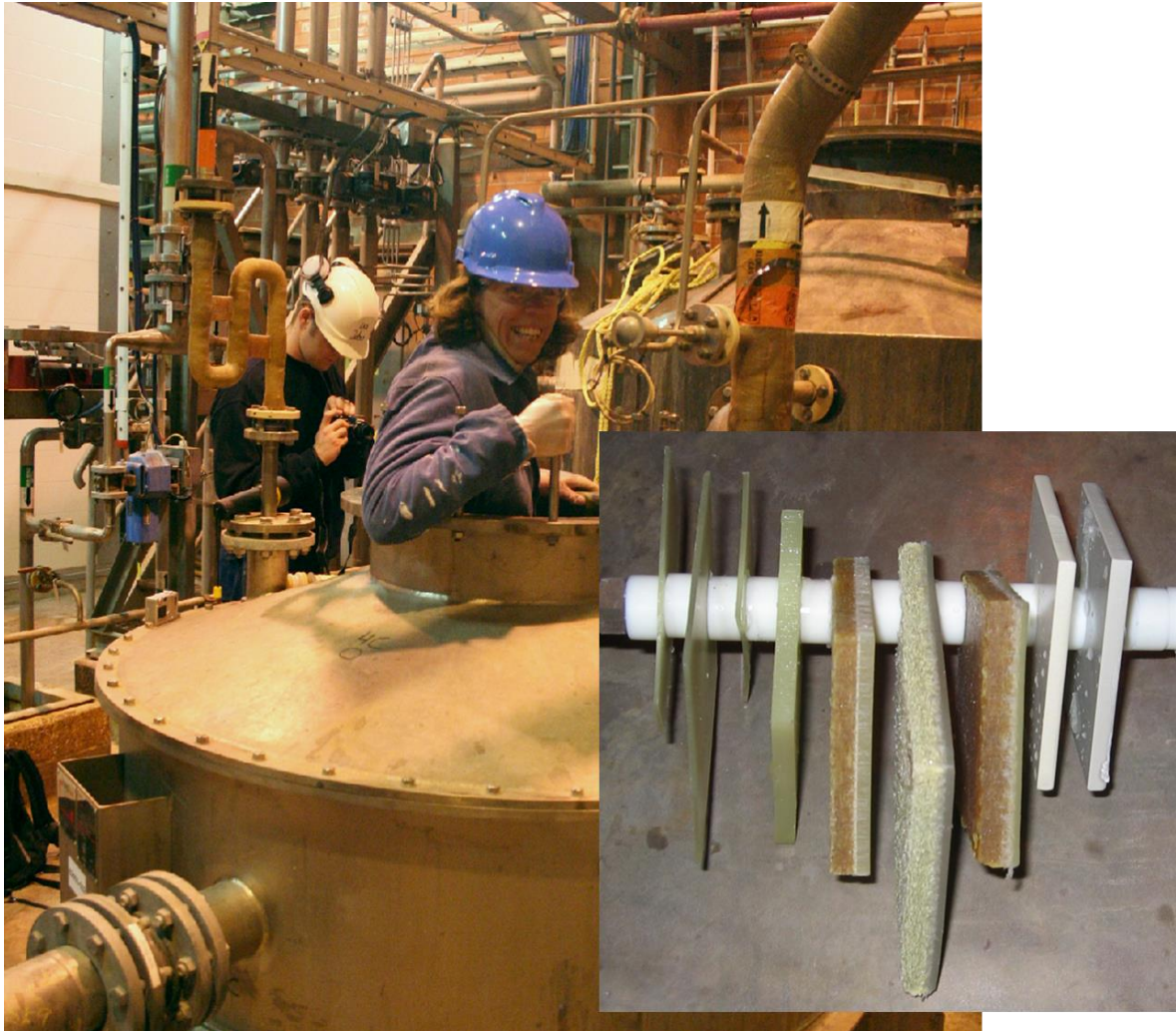
Figure 12. 2005-2008 Swerea KIMAB had a test station in the primary and secondary chlorine dioxide generators at the Skärblacka mill (HP-A)
