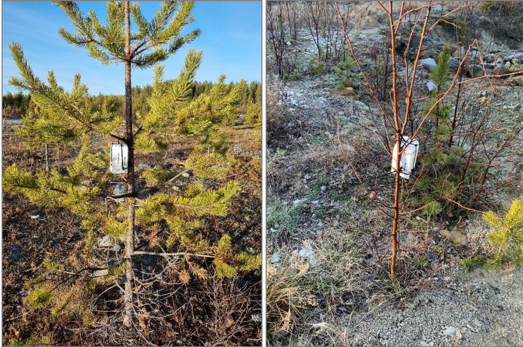
Figure 2 Temperature and humidity loggers in protective housing mounted to nearby trees.
