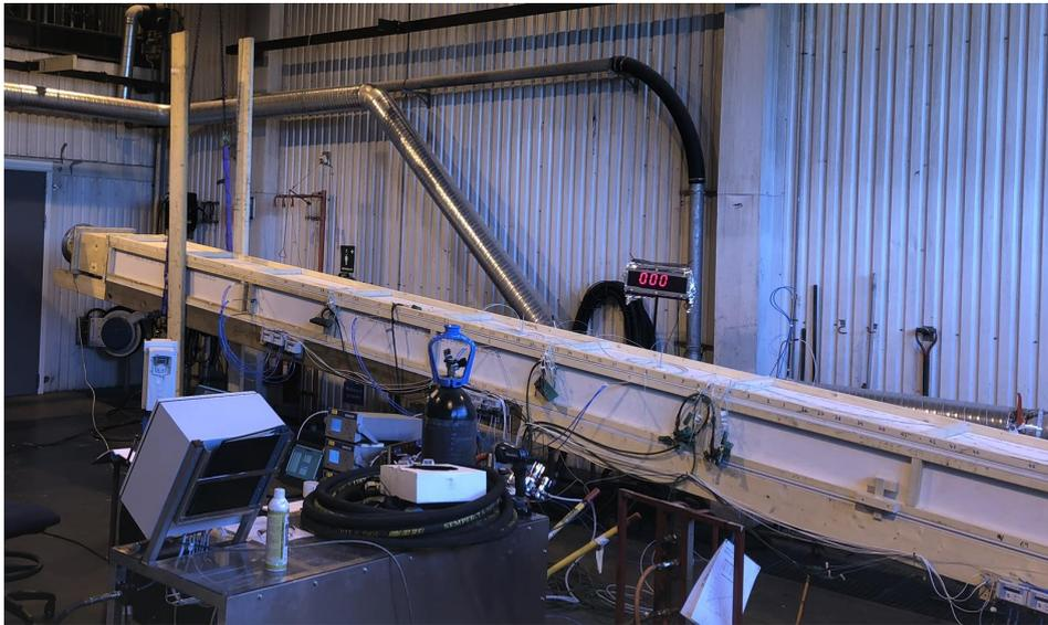
Figure 6. A photo of the model scale tunnel with adjustable slopes (20 % downhill slope).
