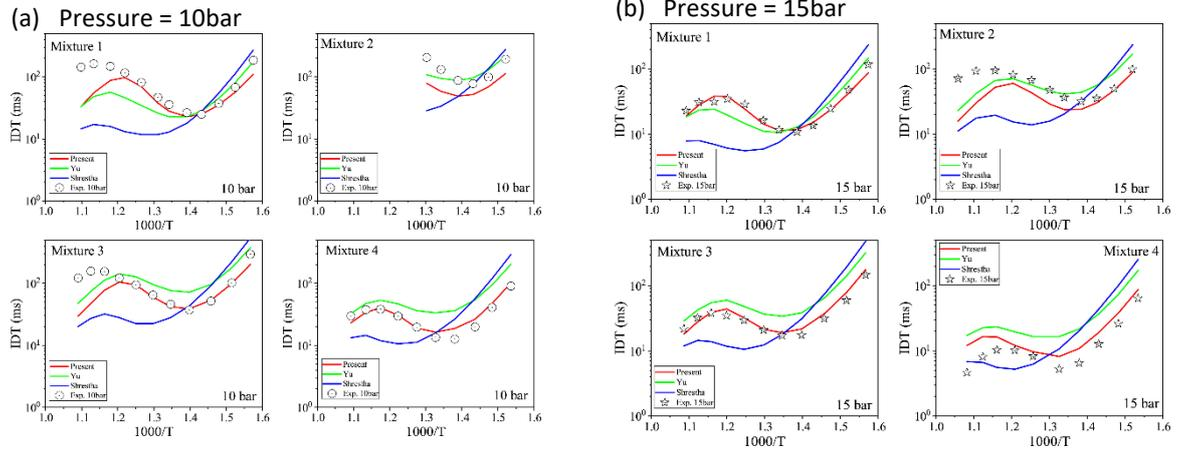
**Fig. 2.** IDTs of n-heptane/NH<sub>3</sub>/O<sub>2</sub>/Ar mixtures at the pressure of 10 bar (a) and 15 bar (b). Symbols are the experimental results and lines are the simulation results using different mechanisms.
