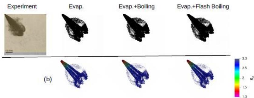
**Fig. 3.** Morphology of ammonia spray liquid phase from different models and experiments and predicted liquid spray morphology colored with the superheat degree  $R_p$  for different conditions.
