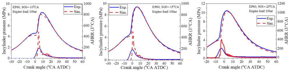
**Figure 7.** In-cylinder pressure and heat release rate with respect to the crank angle for different SOIs under the two engine loads.
