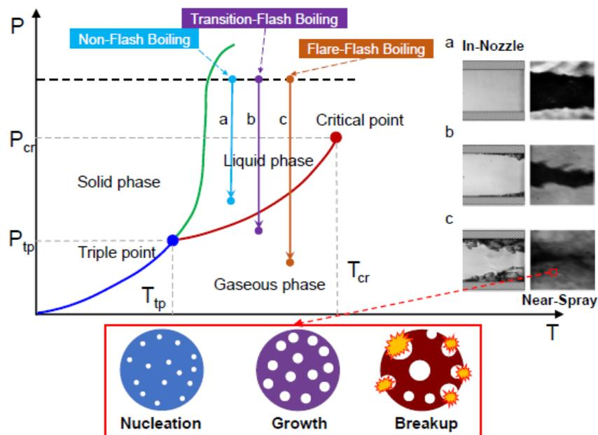
**Fig. 4.** Schematic illustration of the boiling regimes and spray characteristics.
