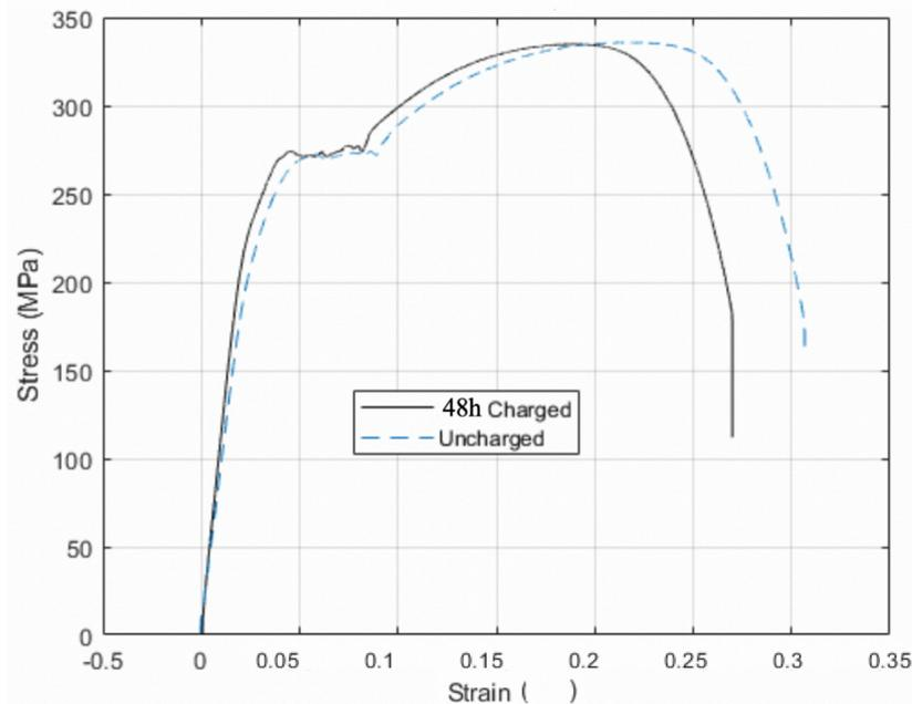
Fig 5. Structural steel specimens with 48h charging time in solid line, and without charged dashed line.
