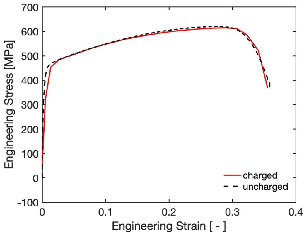
Fig 10. Stress-strain curves of SS321 comparison of results with H2 charged and without charged
