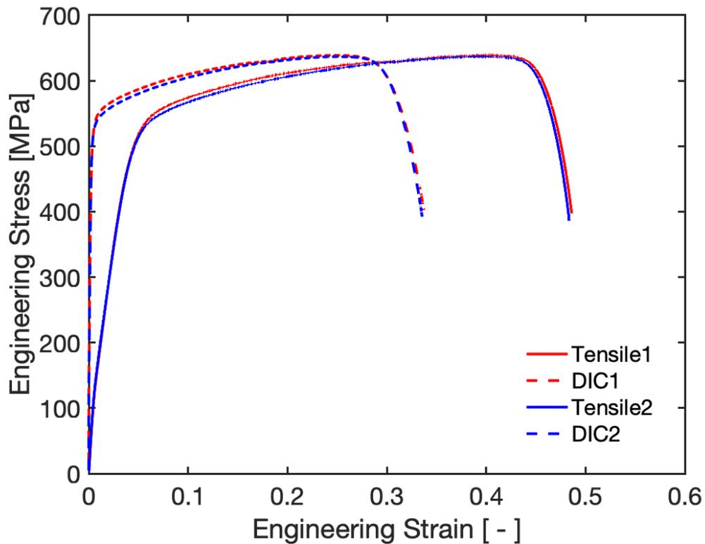
Fig 6. Stress-strain curves of SS304 comparison of results from tensile test measurement vs Correction of strains with DIC measurement
