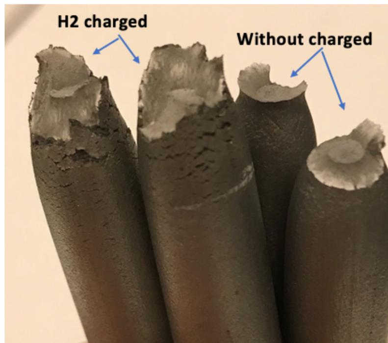
Fig 12 Comparison of fracture surface of SS316L with H2 charged and without charged for slow strain rate (Both tests are performed with slow strain rates, taken with iPhone)
