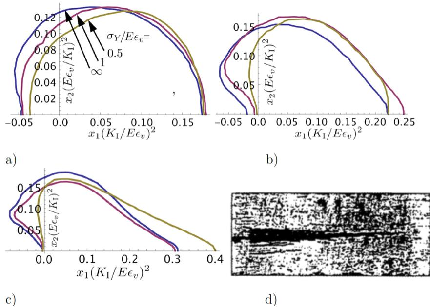
Fig 3. The shape of precipitates for different yield stresses, a) isotropic  $q = 0$  and anisotropic Cases, b) for anisotropy factor  $q = 0.4$ , c) for  $q = 1$ , and d) is a neutron beam scan of a zirconium hydride obtained by Metzger and Sauve [7]. Colour coding is the same in all graphs
