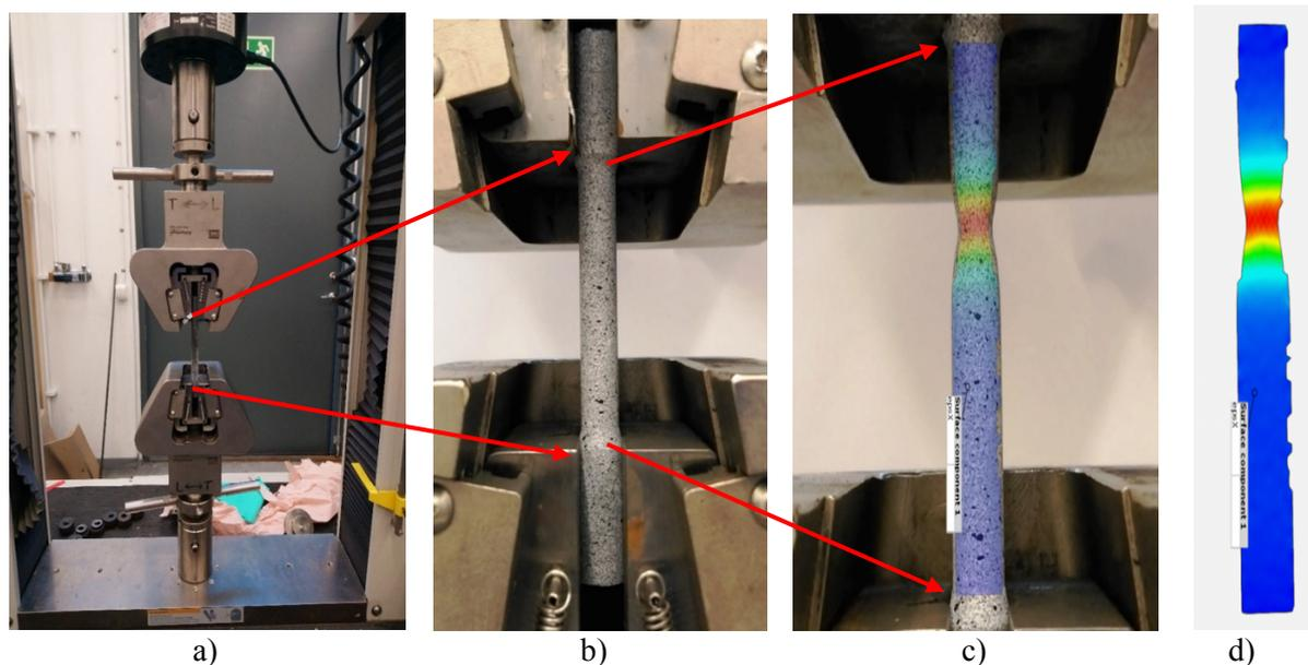
Fig 1. Tensile test of an ASTM cylindrical sample and strain mapping from DIC. From left to right are, a) the grips, b) a typical test specimen with random speckles mounted in the machine, c) a progressive necking with the semi-transparent DIC results, and d) the DIC strain result with red to blue for the highest to the lowest strains.
