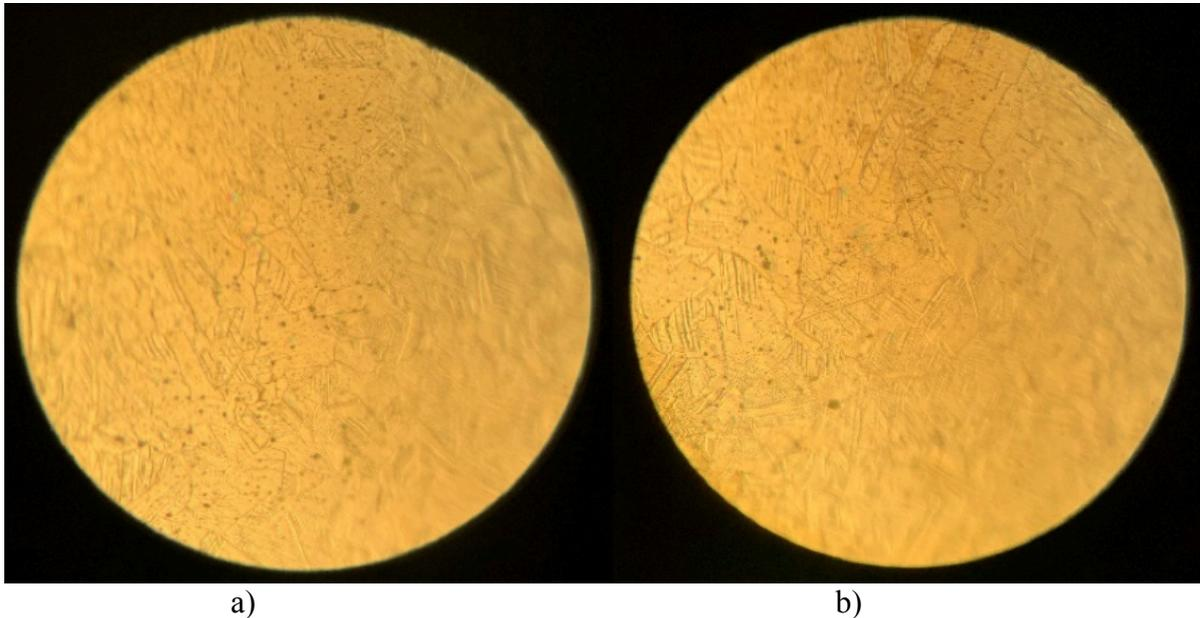
Fig 13. Grain structures a) without charged sample, b) with H<sub>2</sub> charged sample. Samples are taken close around necking region, all with 50x magnification.
