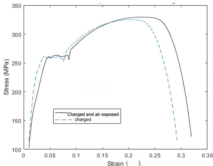
Fig 4. Specimens from structural steel with different transfer time, solid curved is air exposed 8 minutes.
