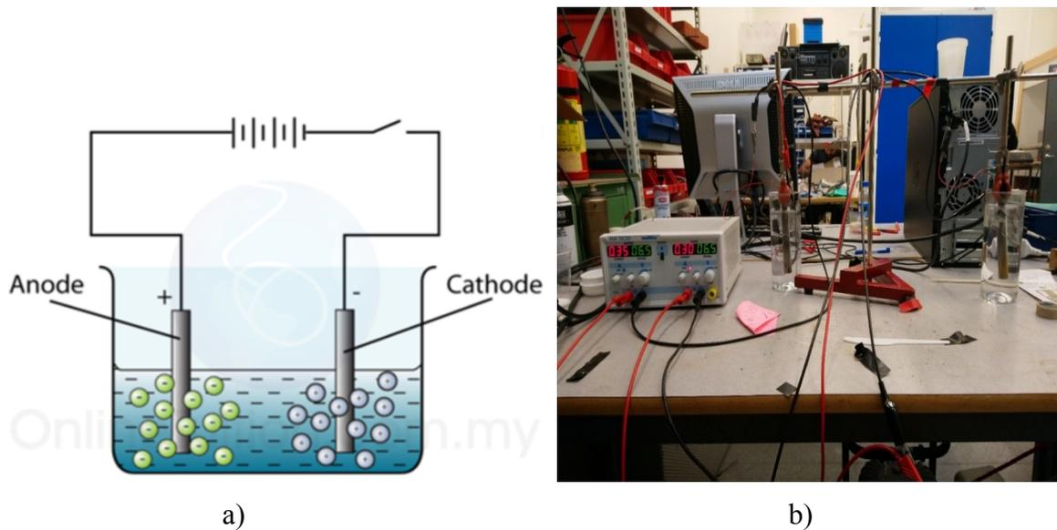
Fig 2. Cathodic charging set up, a) schematic view b) the real setup in the Lab
