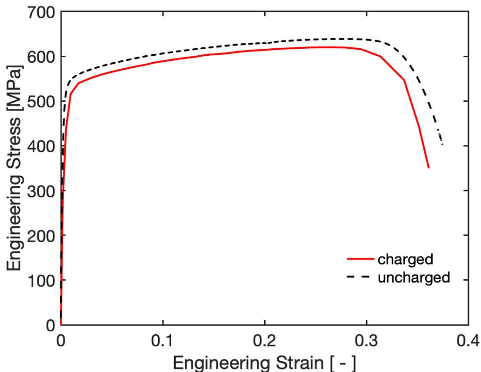
Fig 7. Stress-strain curves of SS304 comparison of results with H<sub>2</sub> charged and without charged specimens
