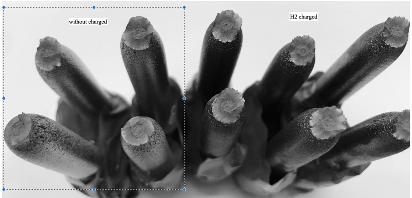
Fig 11 Comparison of fracture surface of SS321, without charged(left, two sets inside frame) and with H2 charged (right, 3 sets)
