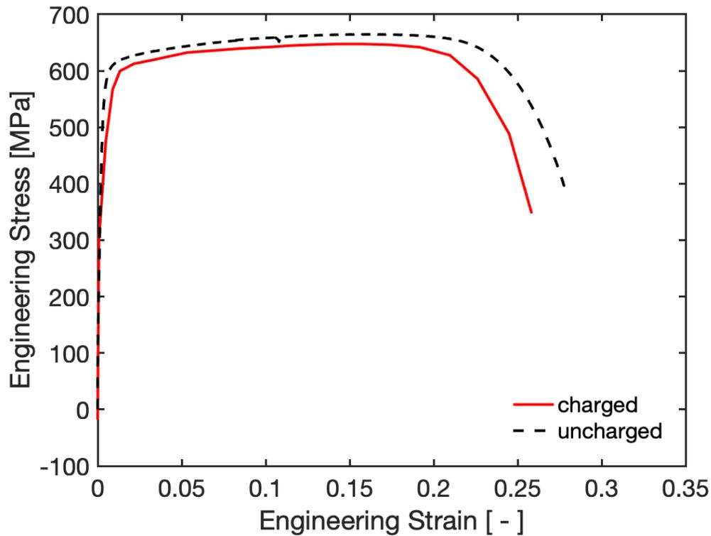
Fig 9. Stress-strain curves of SS316L comparison of results with H2 charged and without charged specimens
