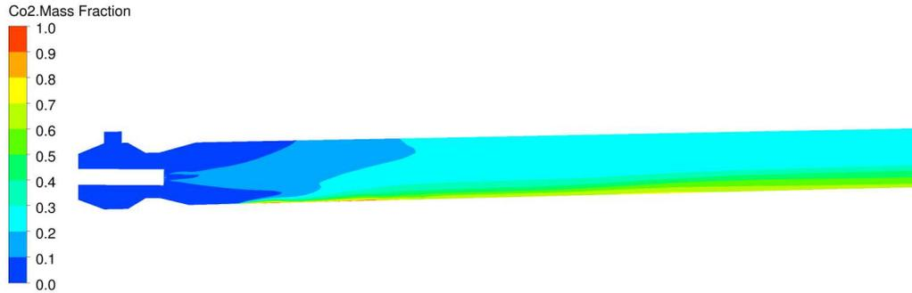
Figure 18 Mass fraction of CO<sub>2</sub> in a cross section along the kiln axis.
