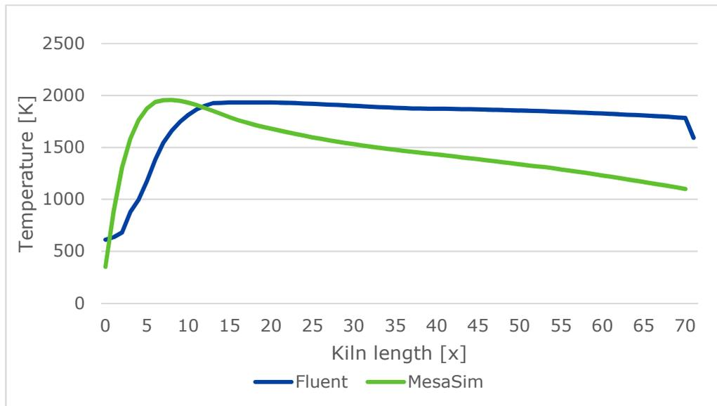
Figure 13 Averaged gas temperature from the CFD simulation compared to the calculated gas temperature from MesaSim.
