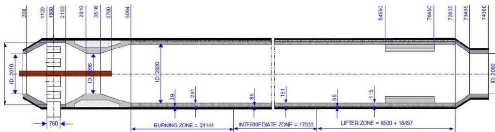
Figure 3 Layout and refractory lining of the Mönsterås lime kiln.
