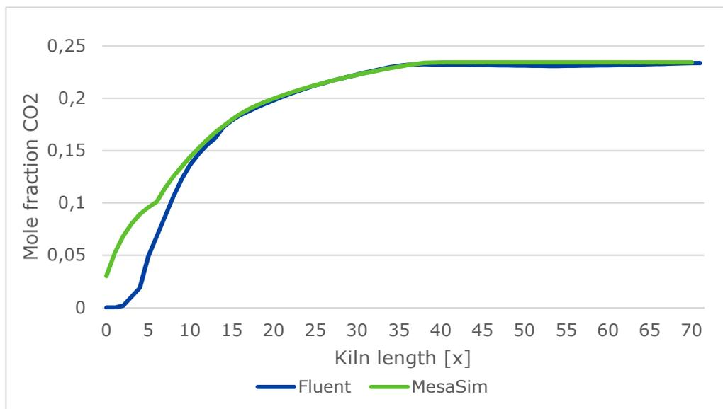
Figure 20 Averaged mass fraction of CO<sub>2</sub> from CFD simulation and MesaSim.
