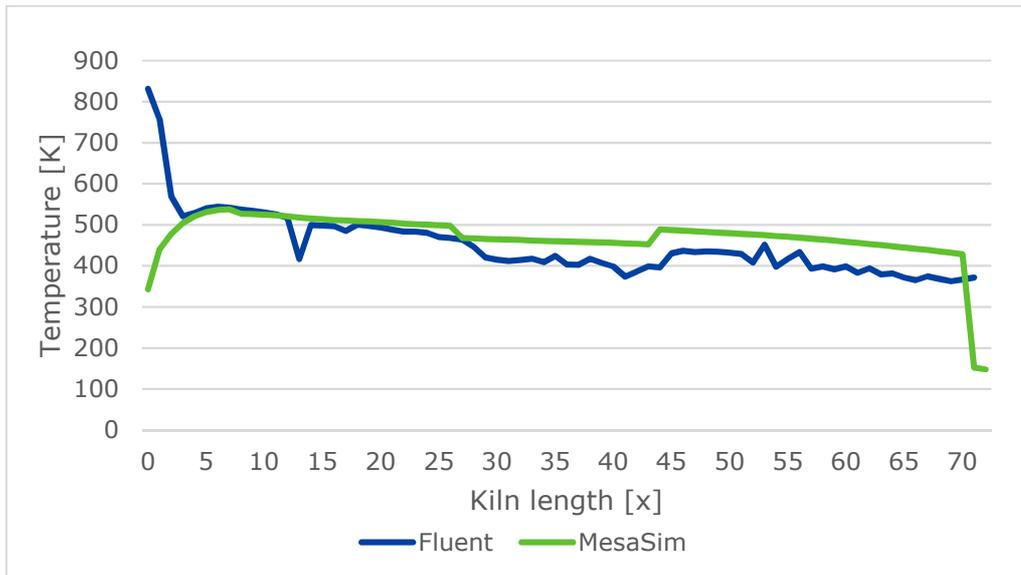
Figure 17 Averaged outer wall temperature from CFD simulation and MesaSim.
