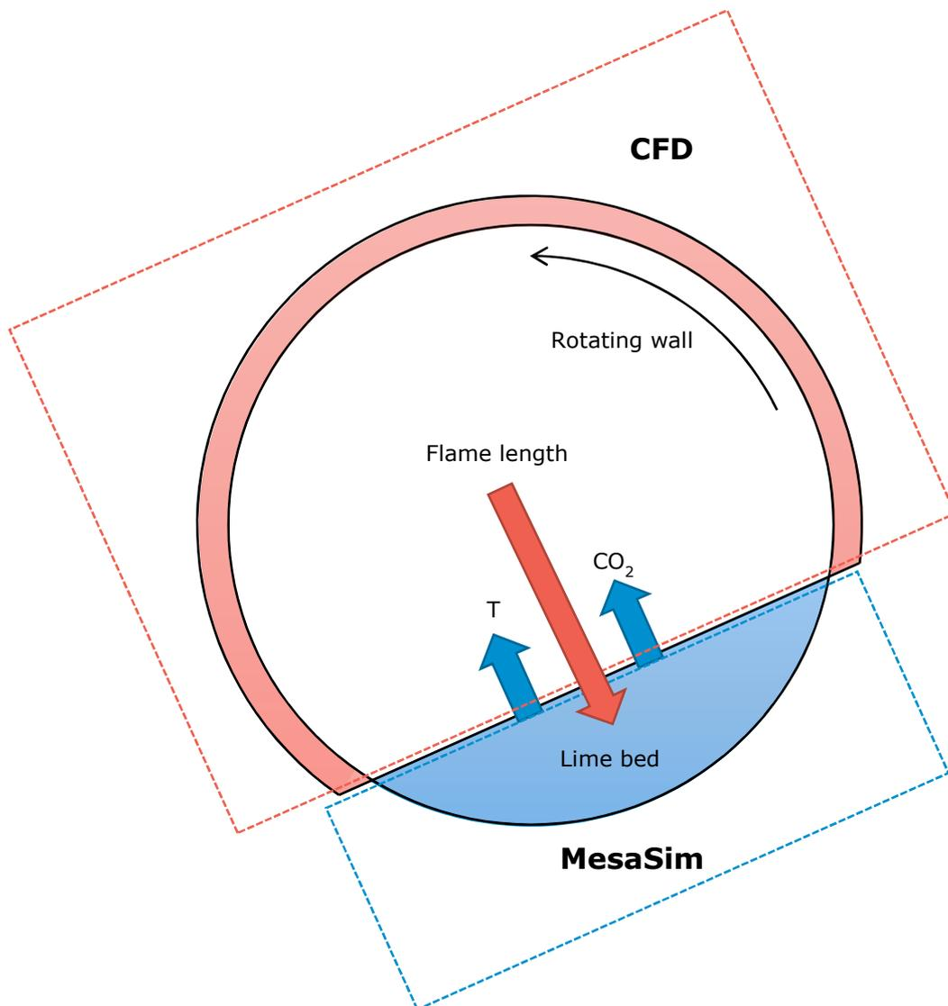
Figure 5 Overview of how the lime kiln is divided between the two models and the information exchange between them.
