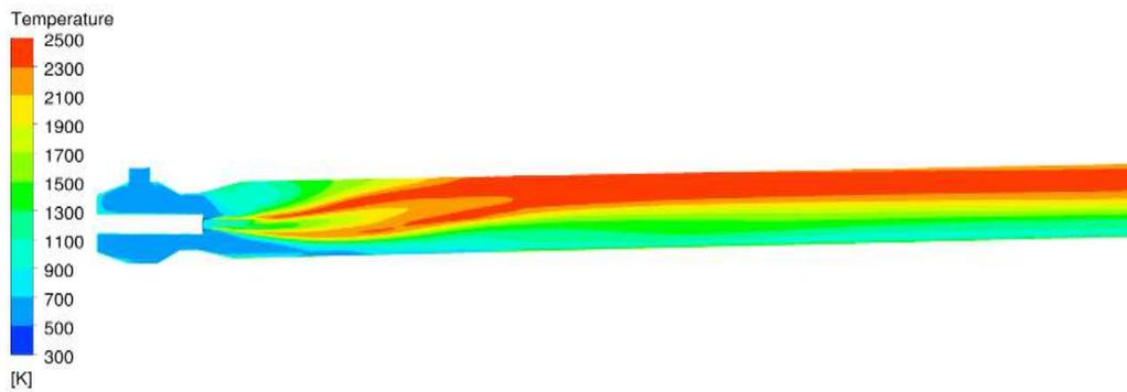
Figure 11 Gas temperature in a cross section along the kiln axis.
