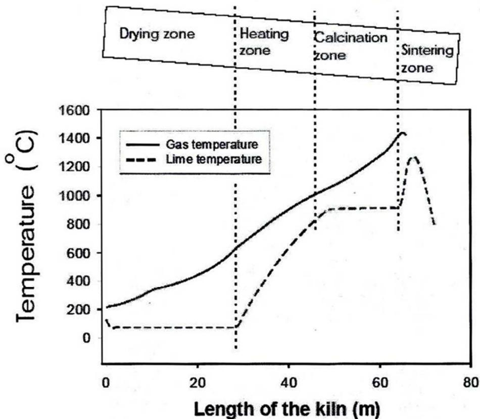
Figure 1 Temperature profile and reaction zones in a rotary lime kiln. causticing process.
