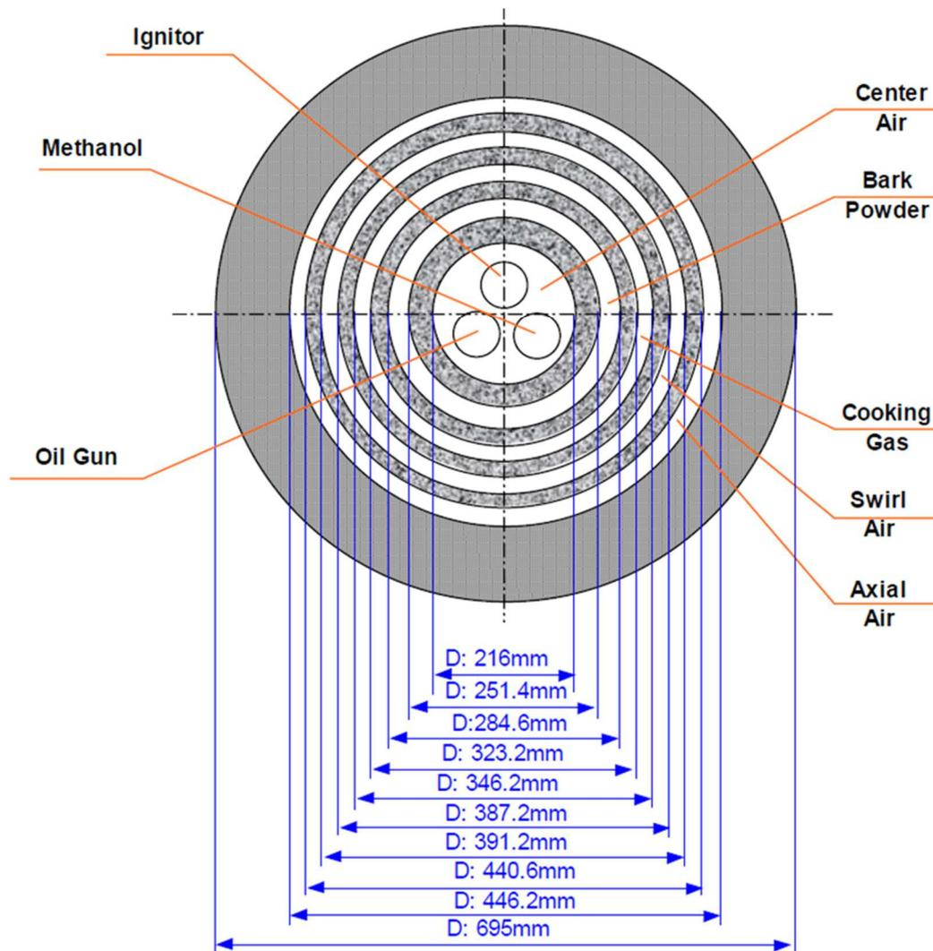
Figure 4 Burner design.
