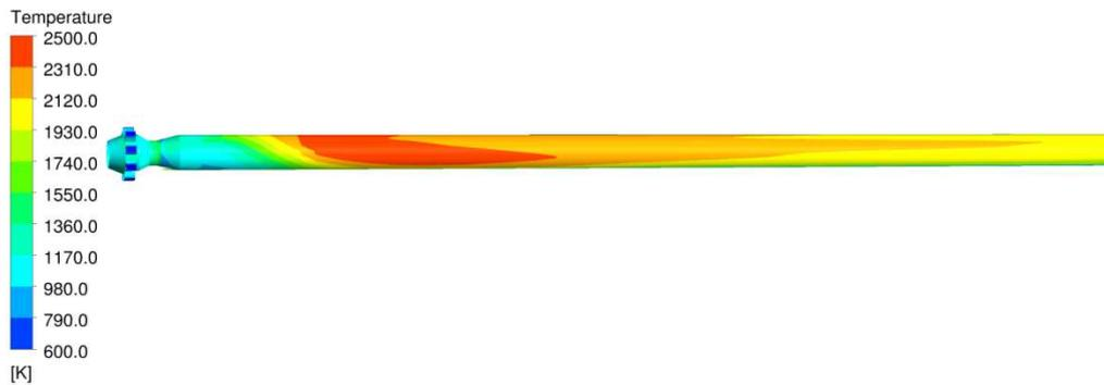
Figure 15 Temperature at the rotating wall on the inside of the kiln.
