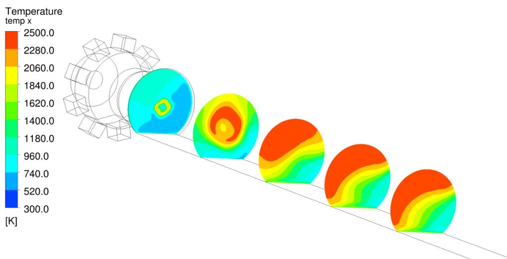
Figure 12 Gas temperature in five cross sections of the kiln ( $x=5, 10, 15, 20, 25m$ ).
