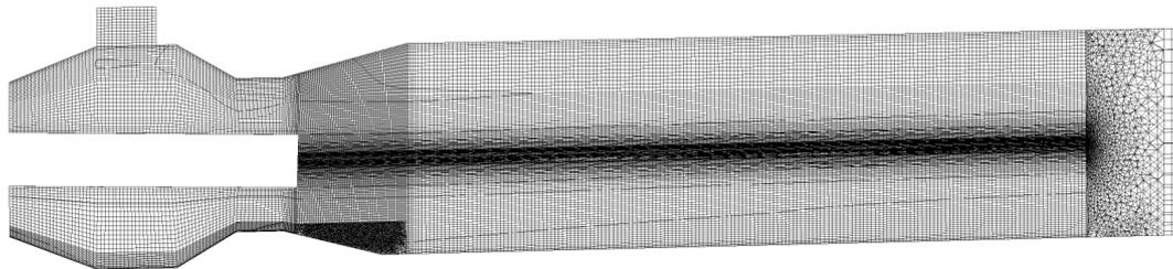
Figure 9 The mesh in the region around the oil burner and air inlets.
