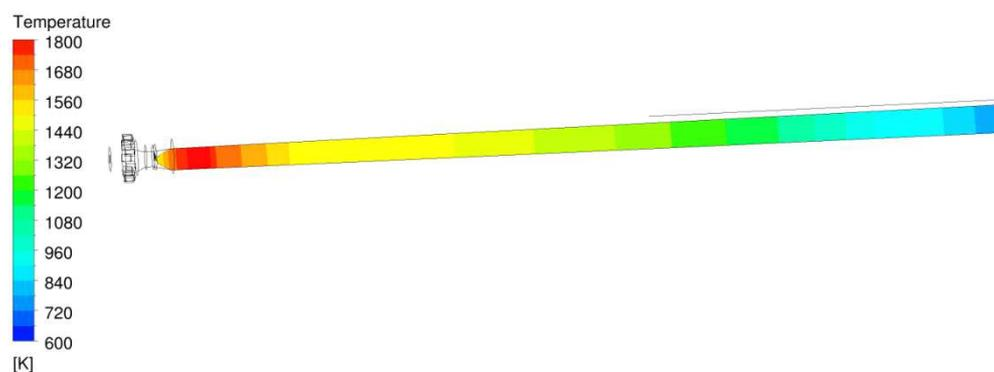
Figure 14 Lime bed temperature calculated in MesaSim and is used as a boundary condition in the CFD model.
