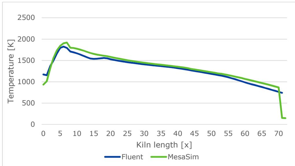
Figure 16 Averaged inner wall temperature from CFD simulation and MesaSim.
