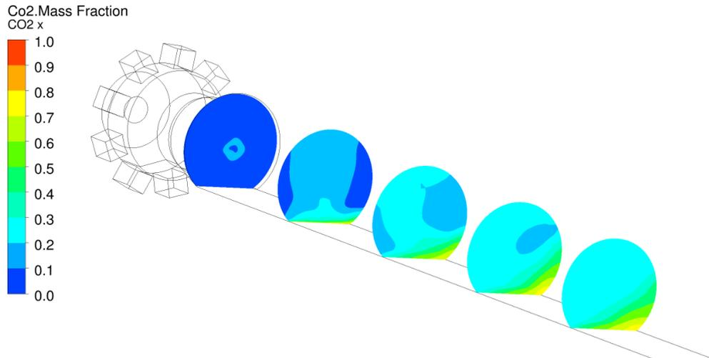
Figure 19 Mass fraction of CO<sub>2</sub> in five cross sections of the kiln ( $x=5, 10, 15, 20, 25m$ ).
