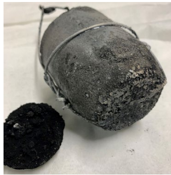
Figure 8 Photo of the molten part of the sample (left) and the crucible (right) after Experiment 3.
